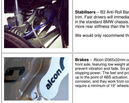
Stabilisers - B3 Anti-Roll Bar Kit complements the chassis balance and trim. Fast drivers will immediately note the prevalent under-steer inherent in the standard BMW chassis. As a consequence we provide significantly more rear stiffness than the front, biasing away from under-steer.
