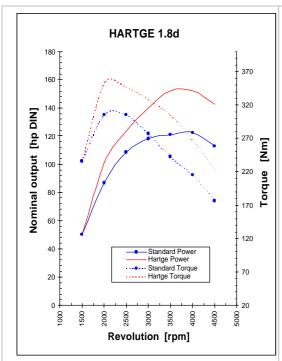
Hartge's Motronic tuning for BMW turbo diesel models were a world first for a major BMW tuner - The result of considerable road and bench testing, the Hartge Motronic Modification system provides a much larger power band, with massive improvements in in-gear acceleration and responsiveness.
