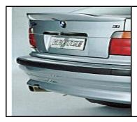
Single Oval Outlet, rear silencer. This rear silencer is available for the E36 Compact 318ti, the E36 Limousine and coupe 328i and also for the E36 M3.
