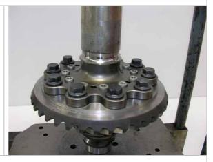
Install LSD gear set into the casing, lubricate bearings with gear oil. Install the left outer race and install the circlip. Press the Quaife gently from the right hand side to ensure the circlip is in the seated position. Install the right outer race and circlip. It may be necessary to press or tap in the right circlip, as this preloads the output bearings.
