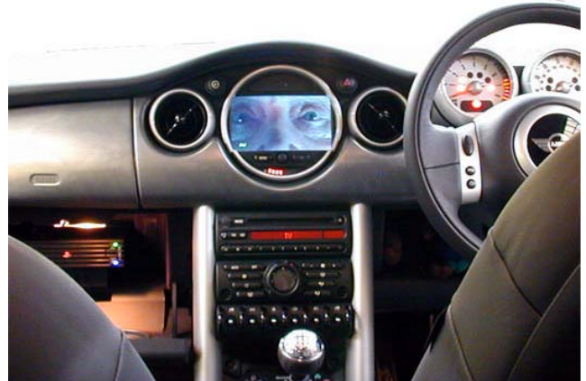
Pictured above is a PS2/DVD driven installation into MINI navigation system.
