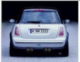
**Sport exhausts** are primarily utilised in maximising the power output from the engine. The standard system is not normally restrictive, but when the performance of the engine is increased, the capacity of the exhaust may be exceeded. We have sport silencers for the Cooper S in two formats;
