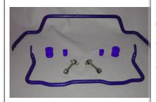
**Stabilisers** – B1 anti-roll bars complement the chassis balance and trim. Fast drivers will immediately note the prevalent under-steer inherent in the standard BMW chassis. As a consequence we provide significantly more rear stiffness than the front, biasing away from under-steer. Again, these stabilisers have been manufactured to our own specifications. These are not off-the-shelf, close-enough items.
