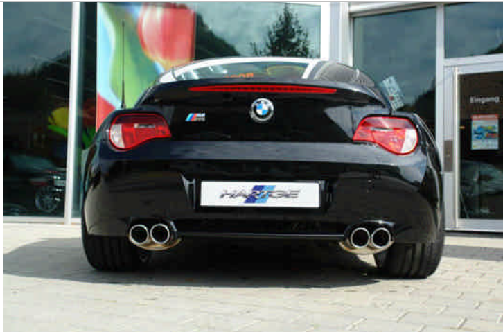
Z4 M Coupe Hartge sport rear silencer with dual round outlets left and right
