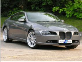
**Body Exterior** - Hartge front spoilers are designed to reduce aerodynamic lift at high speeds, whilst improving cooling to both engine and brakes. Crosswind stability is improved, drag reduced, and the aesthetics of the car dramatically changed.
