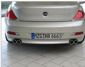
**Sport exhausts** are primarily utilised in maximising the power output from the engine. The standard system is not normally restrictive, but when the performance of the engine is increased, the capacity of the exhaust may be exceeded. The metal catalysts are part of the engine performance kit, and remove the exhaust backpressure, which allows the engine to breath more air, creating more power.
