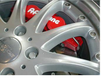
The front brake set can be installed on individually, or in conjunction with the rear brakes. Compatible wheels are standard 17" or 18". Some wheel versions may require adjustment to the wheel offset.
