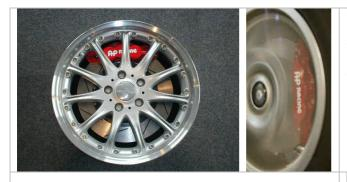
Aluminium alloy six or four opposed piston calipers transmit both the braking force and torque reaction to the chassis. Derived from sports car racing brakes, these have been redeveloped to take into account the harsher environments that road cars have to endure, through salt laden winter roads, and extended service intervals of modern cars.
